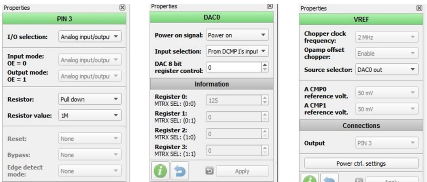
Figure 5. Pin 3, DAC0 and VREF settings
