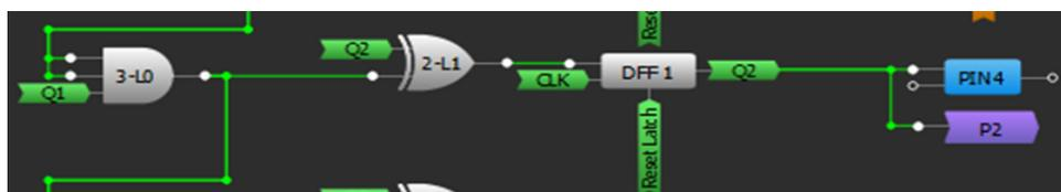
Figure 9. Second Block of 4-Bit Counter
