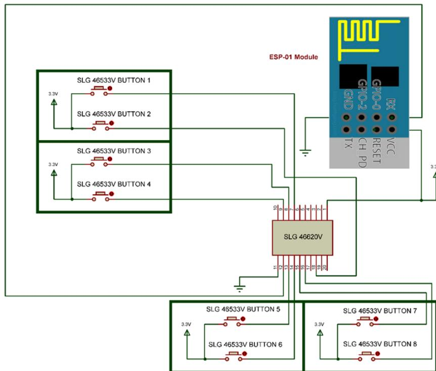
Figure 5. 8 inputs data transmission to ESP-01
