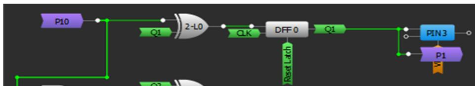
Figure 8. First Block of 4-Bit Counter
