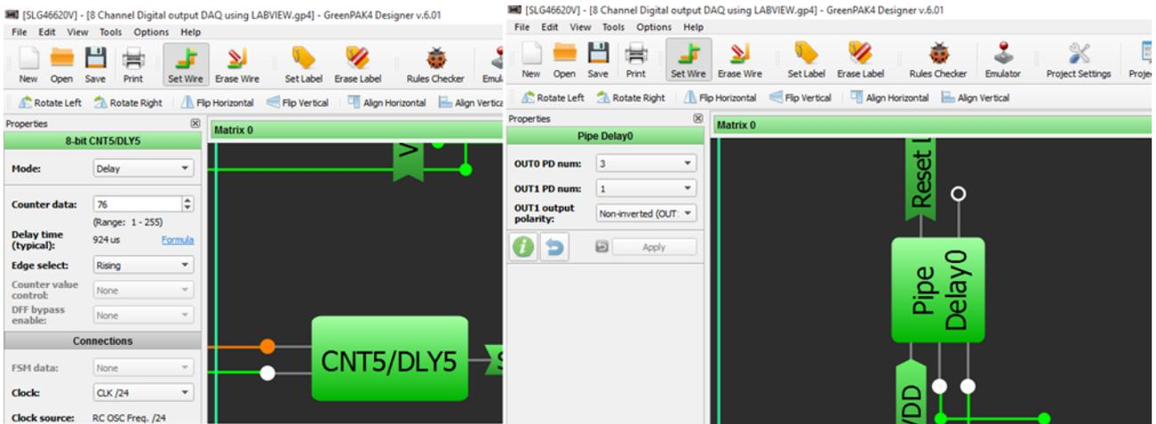
Figure 4. CNT5/DLY5 and Pipe Delay 0 properties
