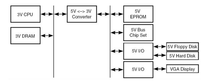
Figure 1. 5V & 3V Logic Mixture in PC Design
