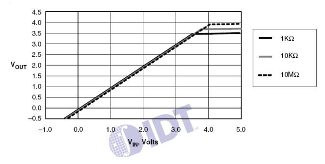
Figure 3. QuickSwitch VOUT vs. VIN
