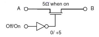
Figure 2. QuickSwitch Block Diagram
