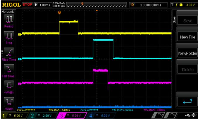
**Figure 10. THROTTLE\_OUT operation when the car has stopped**
