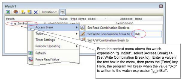
Figure 2.115 Example of Setting a Break Event (Access-related) on a Watch-expression [Simulator]
