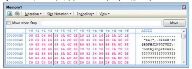
Figure 2.121 Example of Memory Display by the RRM Function (Memory Panel) [E20 (JTAG) [RX600 Series]
