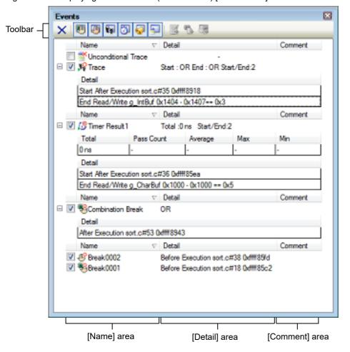
Figure 2.174 Displaying the Set Events (Events Panel) [Simulator]
