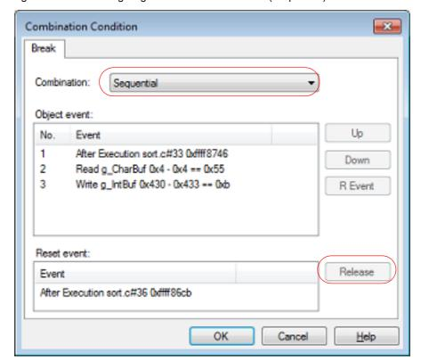
Figure 2.179 Releasing Registration of a Reset Event (Sequential)
