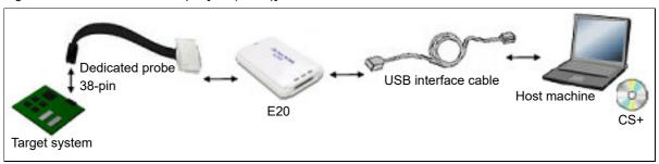
Figure 2.3 Connection Example [E20(Serial)]
