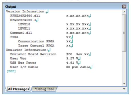
Figure 2.75 Output Panel after Connection [EZ Emulator]
