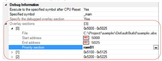
This property shows the current information of overlay sections per address group in detail. Only [Priority section] can be changed.
