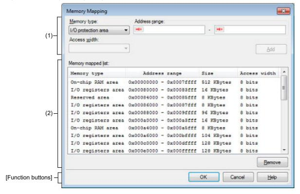
Figure A.24 Memory Mapping Dialog Box [Simulator]
