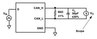
$V_{IN}$  = 125kHz, 0V to  $V_{CC}$ , Duty Cycle 50%,  $t_r = t_f \le 6ns$ ,  $Z_O = 50\Omega C_L$  includes fixture and instrumentation capacitance.
