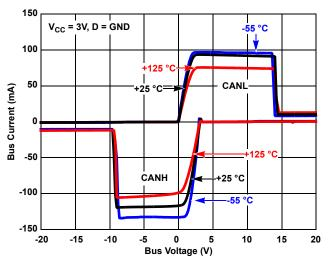
Figure 40. Driver Output Current vs Short-Circuit Voltage vs Temperature
