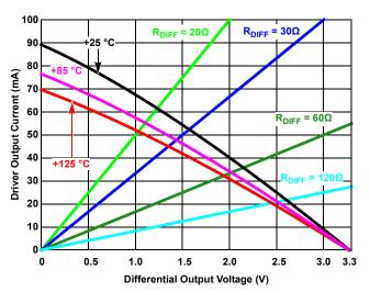
Figure 39. Driver Output Current vs Differential Output Voltage
