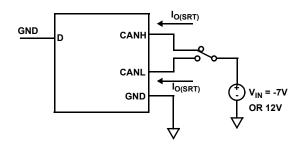
Figure 24. Output Short-Circuit Current Test Circuit
