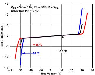
Figure 31. Bus Pin Leakage vs ±35V VCM
