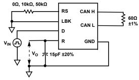
$V_{IN}$  = 125kHz, Duty Cycle 50%,  $t_r = t_f \le 6ns$ .
