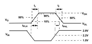
Figure 17. Receiver Test Measurement Points
