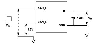
$V_{IN}$  = 125kHz, Duty Cycle 50%, t<sub>r</sub> = t<sub>f</sub> = 6ns, Z<sub>O</sub> = 50 $\Omega$ C<sub>L</sub> includes test setup capacitance
