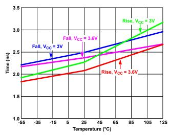
Figure 45. Receiver Rise and Fall Times vs Temperature
