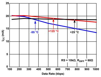
Figure 27. Supply Current vs Medium Data Rate vs Temperature
