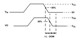
$V_{\text{IN}}$  = 125kHz, 0V to  $V_{\text{CC}},$  Duty Cycle 50%,  $t_{r}$  =  $t_{f}$   $\leq$  6ns
