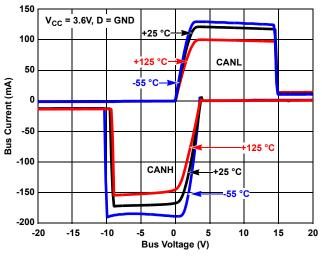
Figure 41. Driver Output Current vs Short-Circuit Voltage vs Temperature
