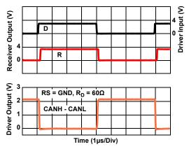
Figure 2. Fast Driver and Receiver Waveforms
