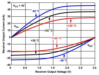
Figure 42. Receiver Output Current vs Receiver Output Voltage at  $V_{CC}$  = 3V
