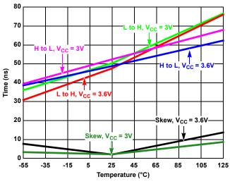
Figure 44. Receiver Propagation Delay and Skew vs Temperature
