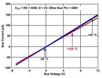
Figure 29. Bus Pin Leakage vs VCM at  $V_{CC}$  = 0V
