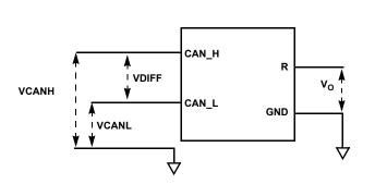
Figure 15. Receiver Voltage Definitions
