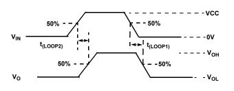
Figure 21. Total Loop Delay Measurement Points
