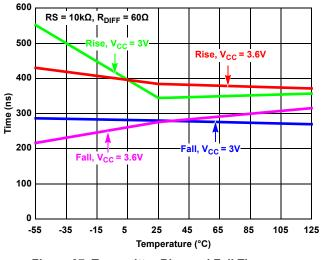
Figure 37. Transmitter Rise and Fall Times vs Temperature at Medium Speed
