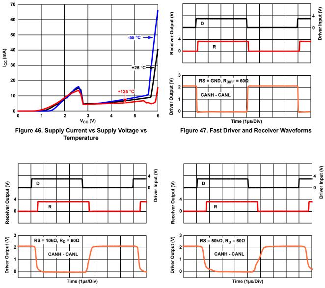
Figure 48. Medium Driver and Receiver Waveforms
