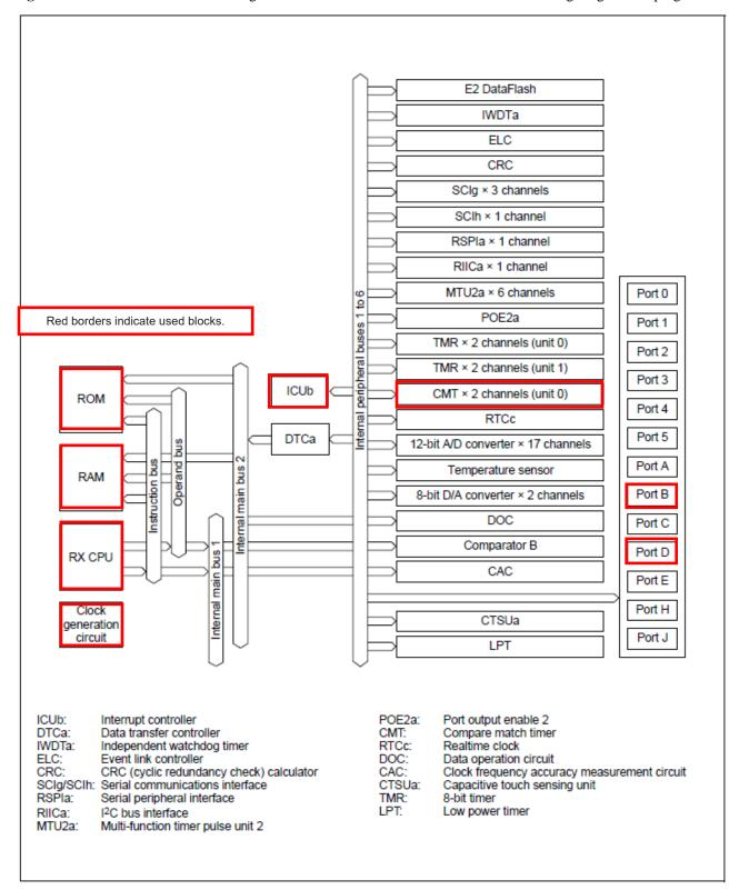
Figure 3-1: RX130 Internal block diagram
