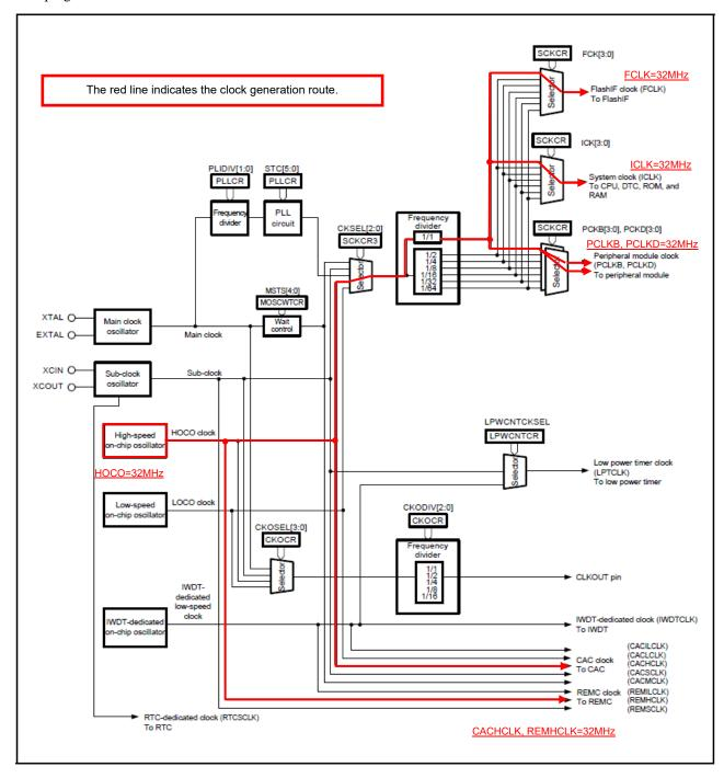
Figure 5-1: RX130 Clock generation block diagram
