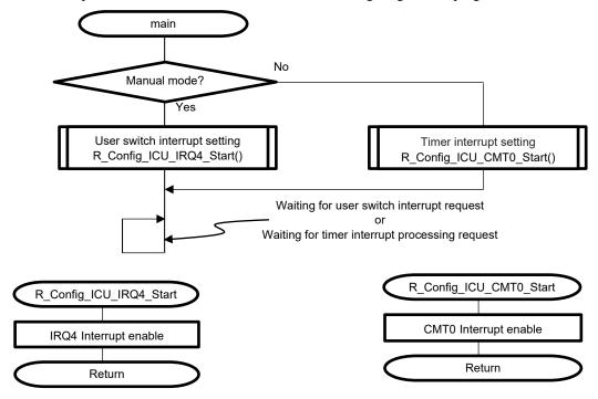
Figure 2-2: LED lighting control program operation flow
