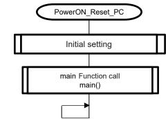
Figure 2-1: Power-on reset operation flow
