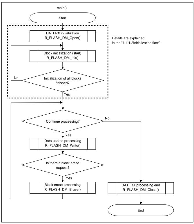
Figure 1.2 Processing Example of Main Function (Flash Type 1)
