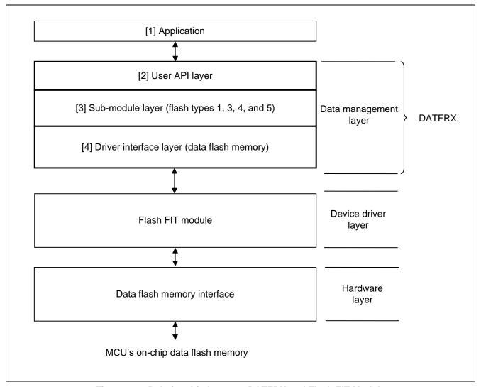
Figure 1.1 Relationship between DATFRX and Flash FIT Module
