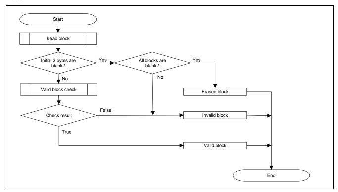
Figure 5.4 Block State Determination Flowchart (Flash Types 3, 4, and 5)
