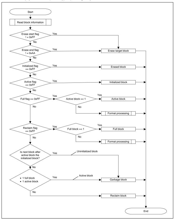
Figure 5.2 Block State Determination Flowchart (Flash Type 1)
