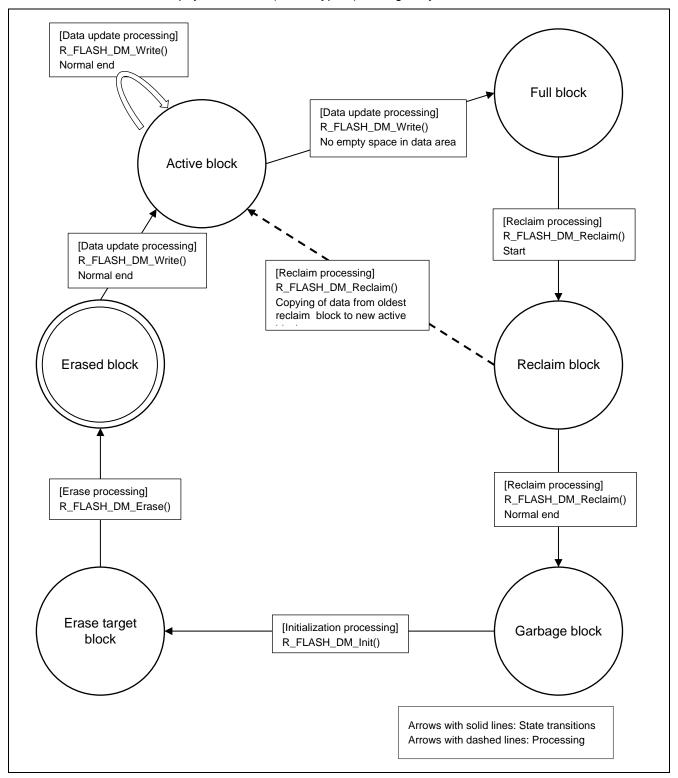
Figure 5.1 Block State Transitions (Flash Type 1)
