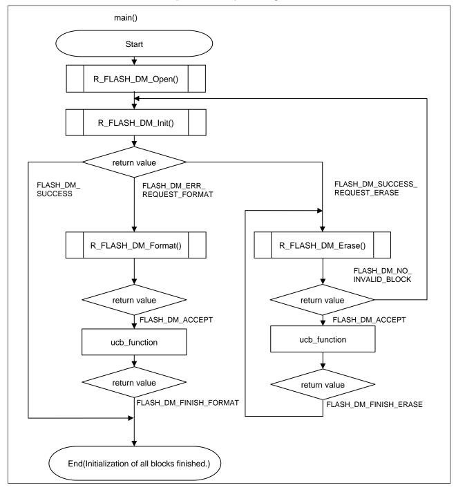
Figure 1.3 Example of processing after R\_FLASH\_DM\_Init() (Flash Type 1)
