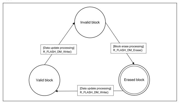
Figure 5.3 Block States (Flash Types 3, 4, and 5)
