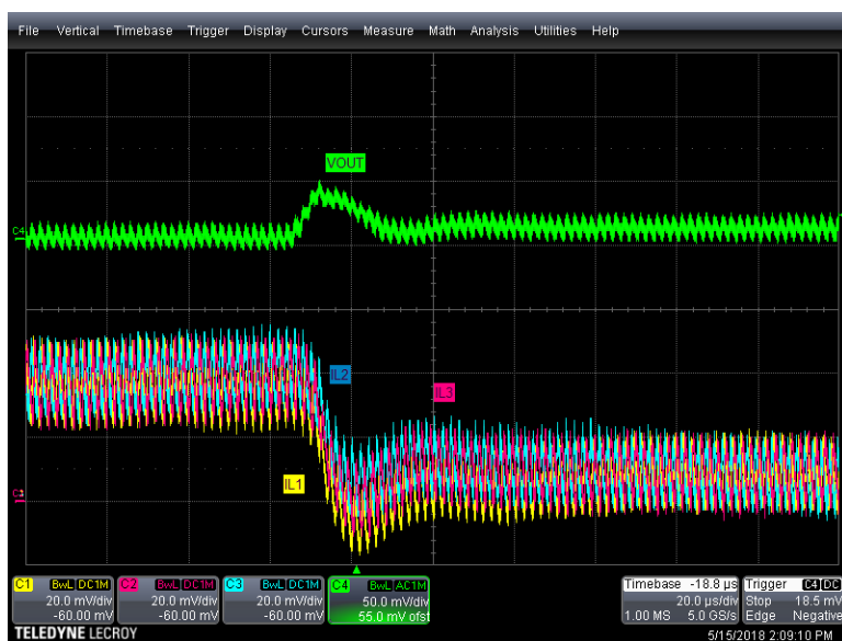
Figure 6: Current sharing during load release
