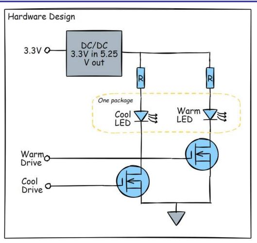
We will drive the two transistor gates with the output from a PWM running with a carrier frequency of 4kHz. This is well above the optical detection of the eye – even in the periphery where we are more sensitive, and well below where the switching transitions occupy a high percentage of overall time (this, in the end, is what makes transistors run hot – not what percentage of time they are on, but the percentage of time they spend in the linear region during switching).
