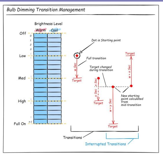
As you can see, because of my need to do smooth dimming, there is the possibility that a command can interrupt a dimming in progress, so in that case the dimming "path" will be more than the 100 steps between settings. But it will eventually settle on the correct value.
