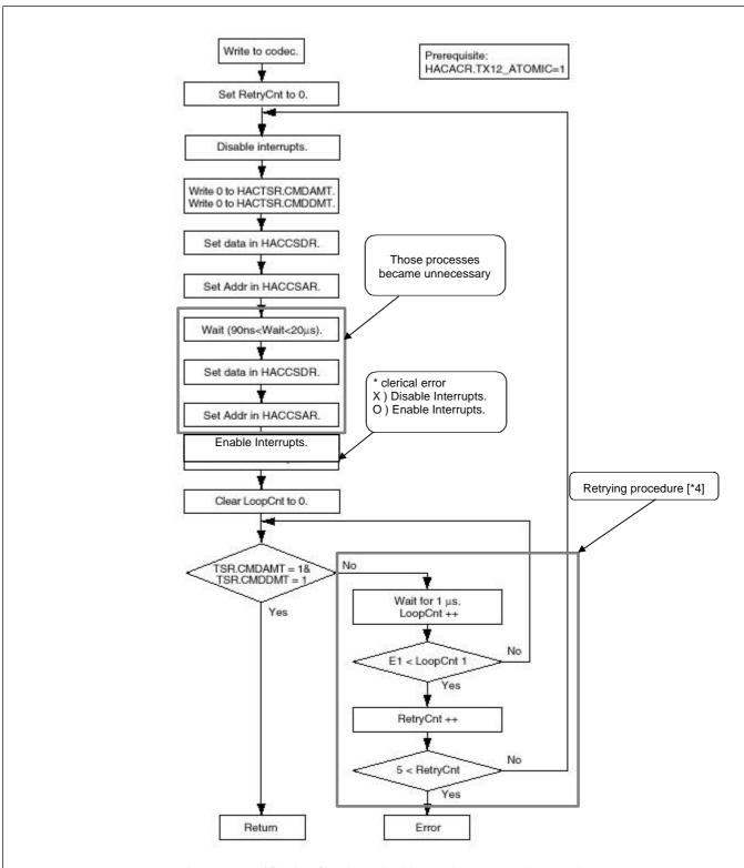
Figure 1. Modification for Figure 25.4 in Hardware Manual Rev 1.0
