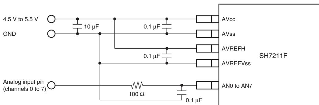
Page 792, 17.7.7 Treatment of AV<sub>CC</sub> and AV<sub>SS</sub> When the A/D Converter is Not Used is added as follows.
