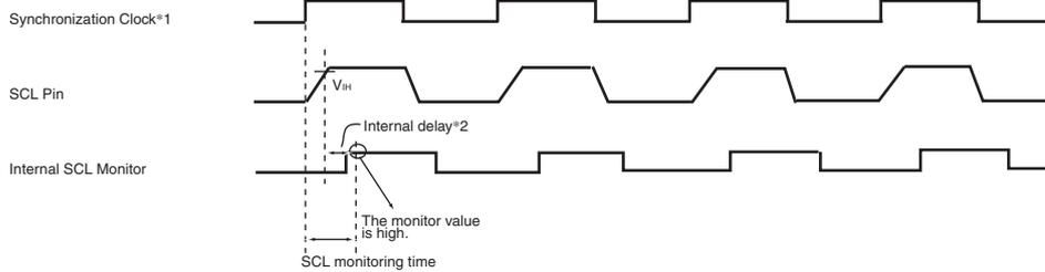
(2) When the period in which the slave device outputs low is extended
