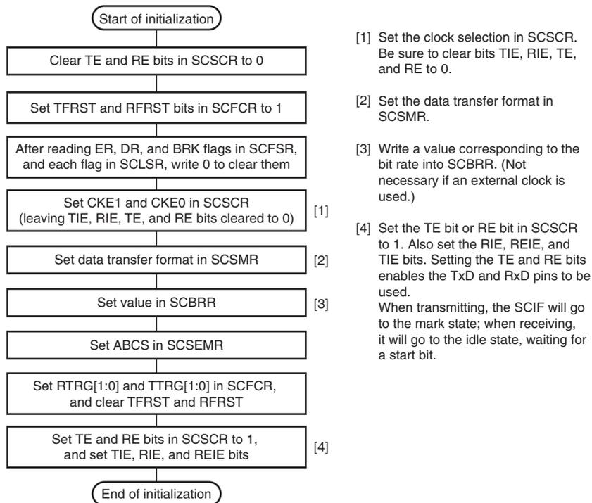
Page 715, Figure 15.11 Sample Flowchart for Transmitting Serial Data
