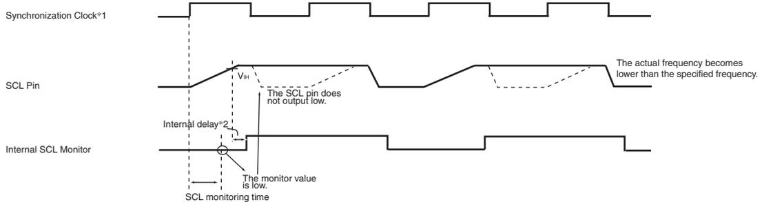
Notes: 1. A clock whose transfer rate is specified by the CKS[3:0] bits in the I2C bus control register (ICCR1).
