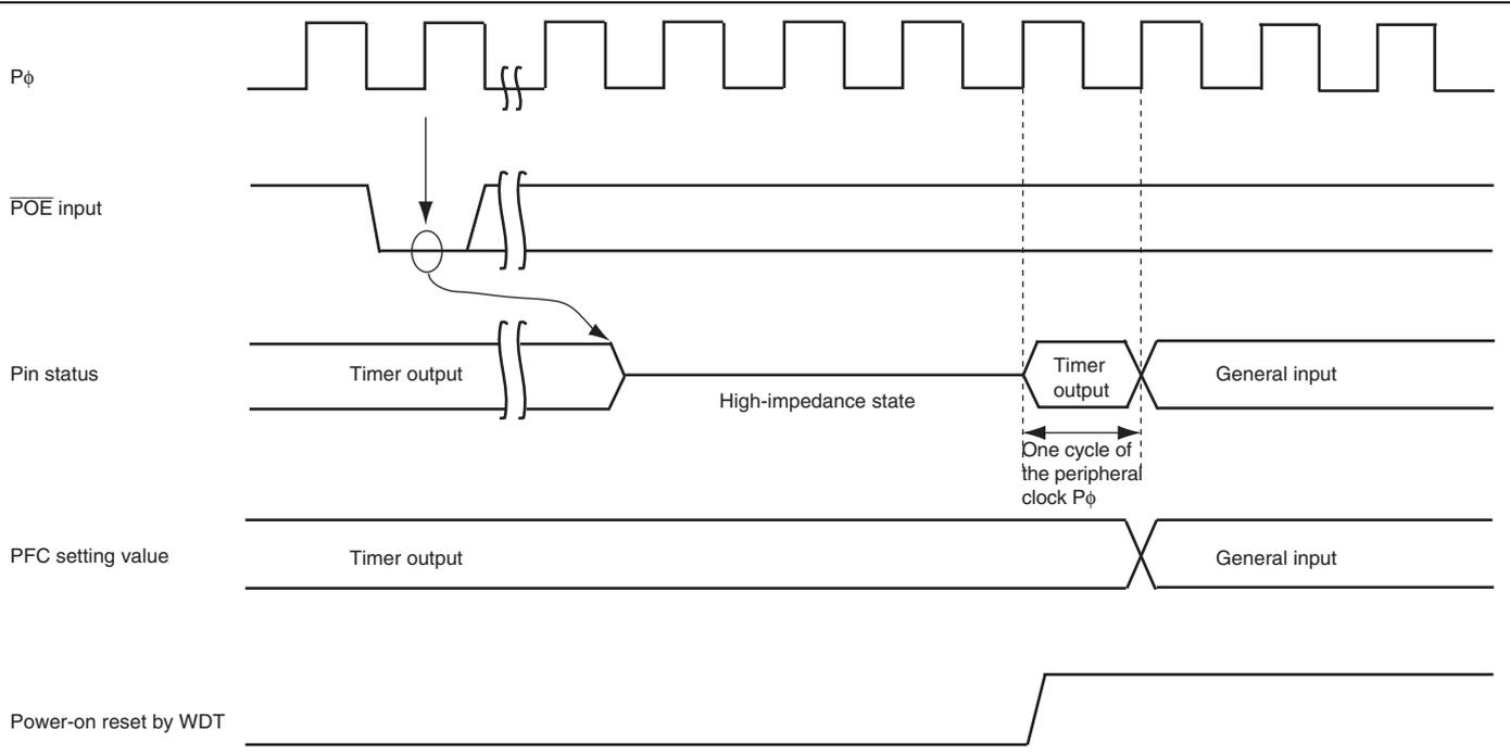
Figure 12.5 Pin Status When Power-on Reset Is Issued from Watchdog Timer
