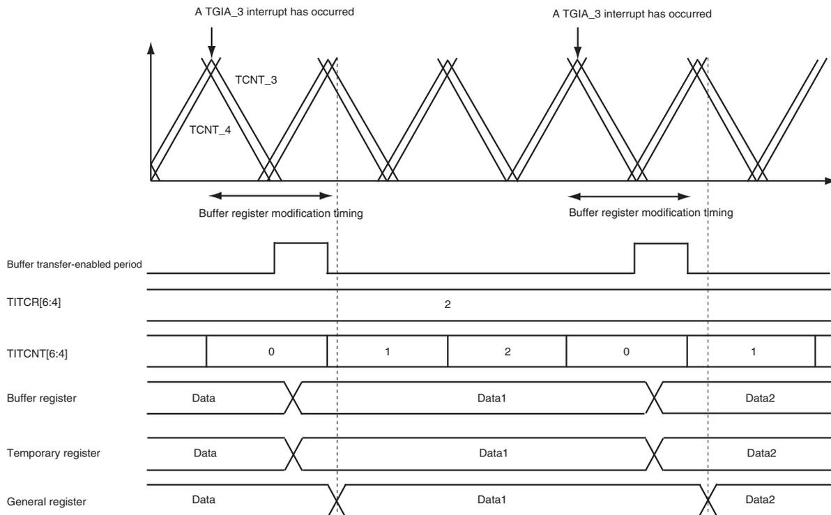
(2) When the buffer register is modified after one carrier cycle has been passed from a TGIA\_3 interrupt occurrence
