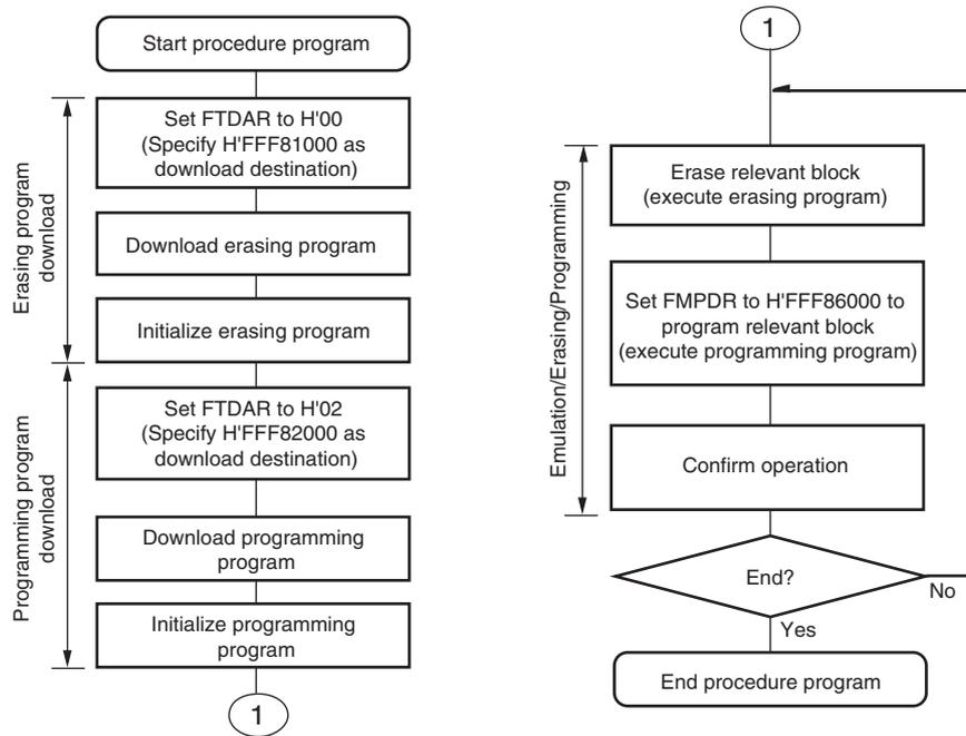
Page 933, (4) Erasing and Programming Procedure in User Program Mode, 2. Be sure to initialize both the erasing program and programming program.
