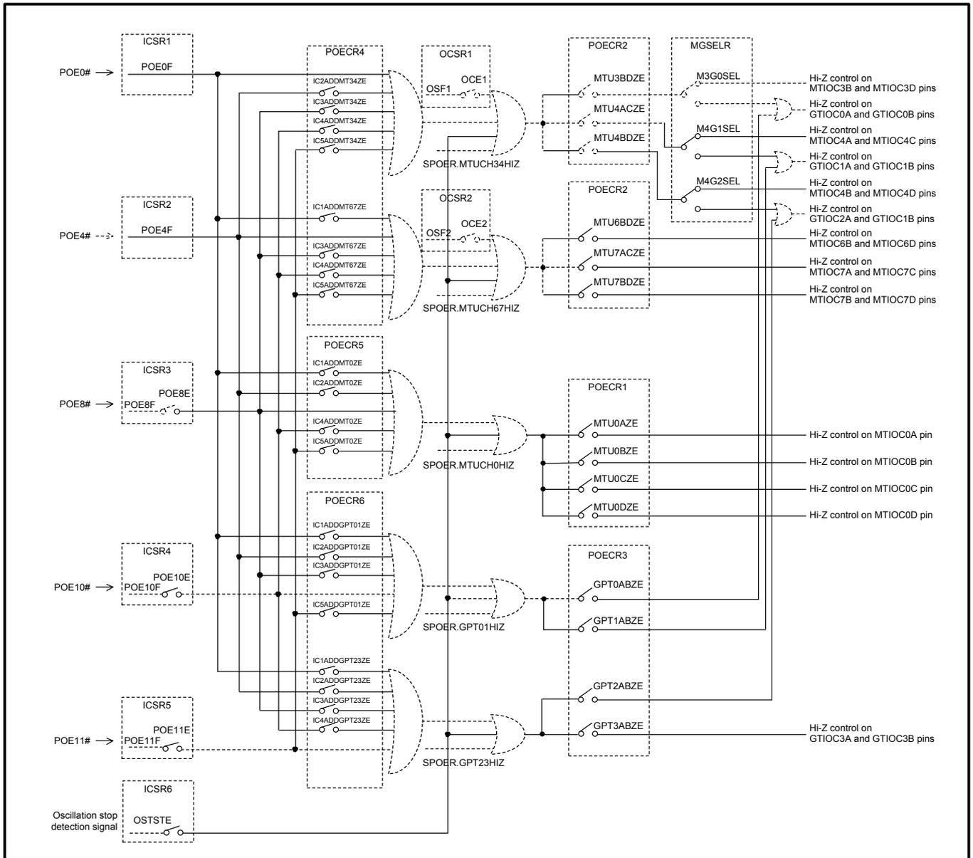
Figure 25.2 Target Pins and Conditions for High-Impedance Control
