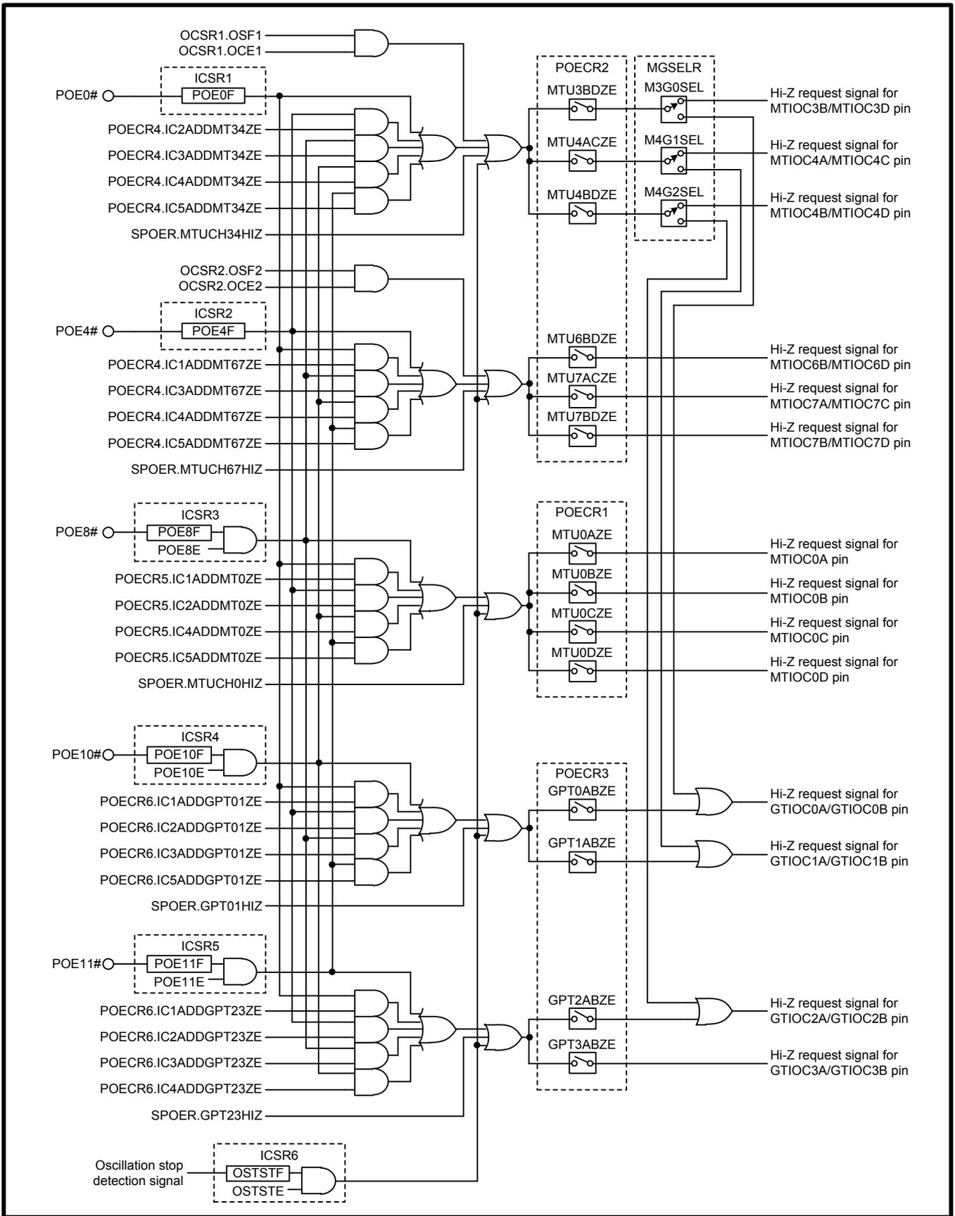
Figure 25.2 Target Pins and Conditions for High-Impedance Control
