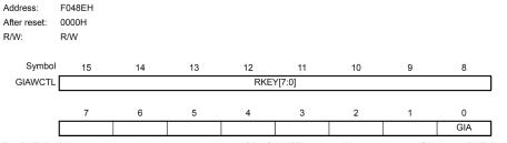
The RKEY[7:0] bits contain the key code to control rewriting of the GIAWCTL register. When rewriting the GIA bit, set RKEY[7:0] to **C4H** and then write to all 16 bits of this register at once. The RKEY[7:0] bits return 00H when read.
