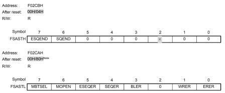
Note The initial value of the MBTSEL bit is undefined because it depends on the value of the BTFLG bit (boot area switching flag) stored in the extra area.
