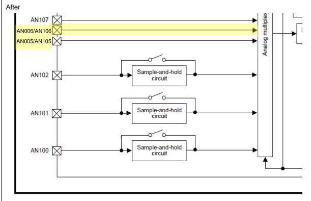
Figure 45.2 ADC12 unit 1 block diagram
