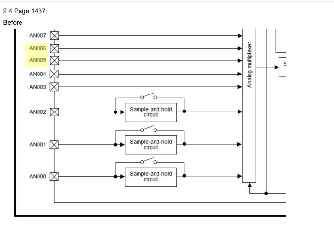
Figure 45.1 ADC12 unit 0 block diagram
