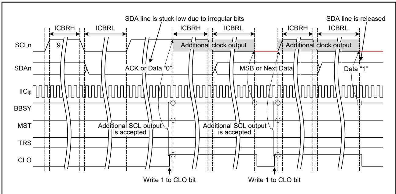
**Figure 31.40 Additional SCL Output Function (CLO Bit)**
