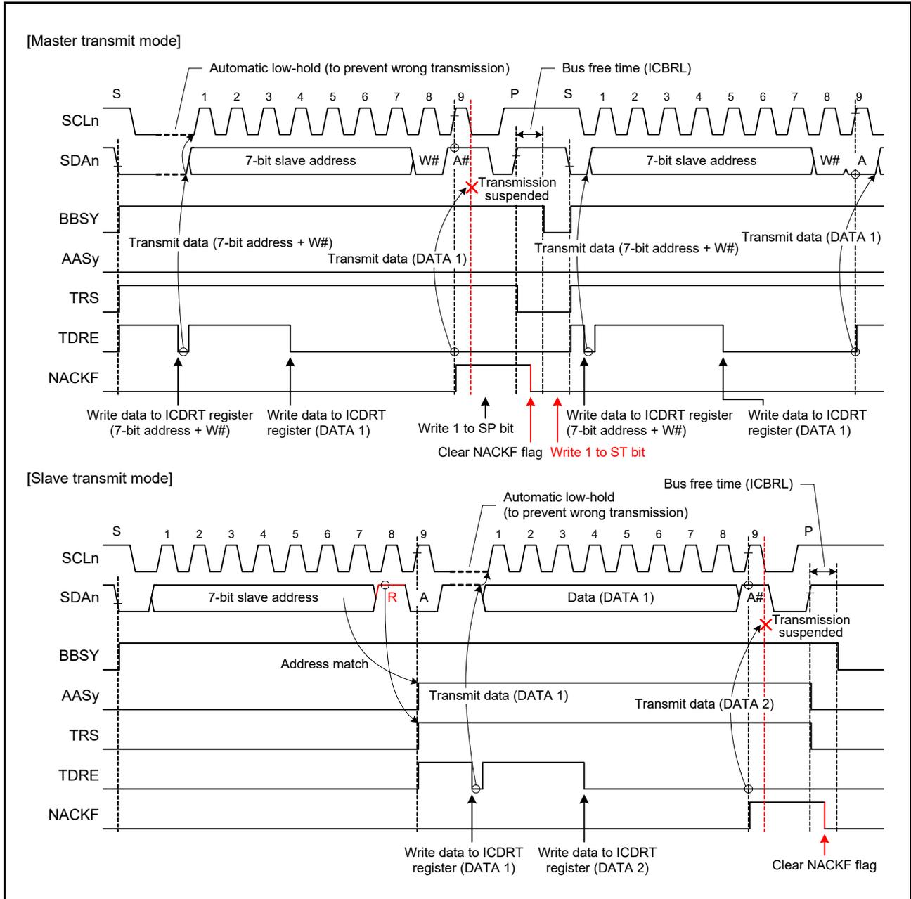
Figure 31.31 Suspension of Data Transmission When NACK is Received (NACK = 1)
