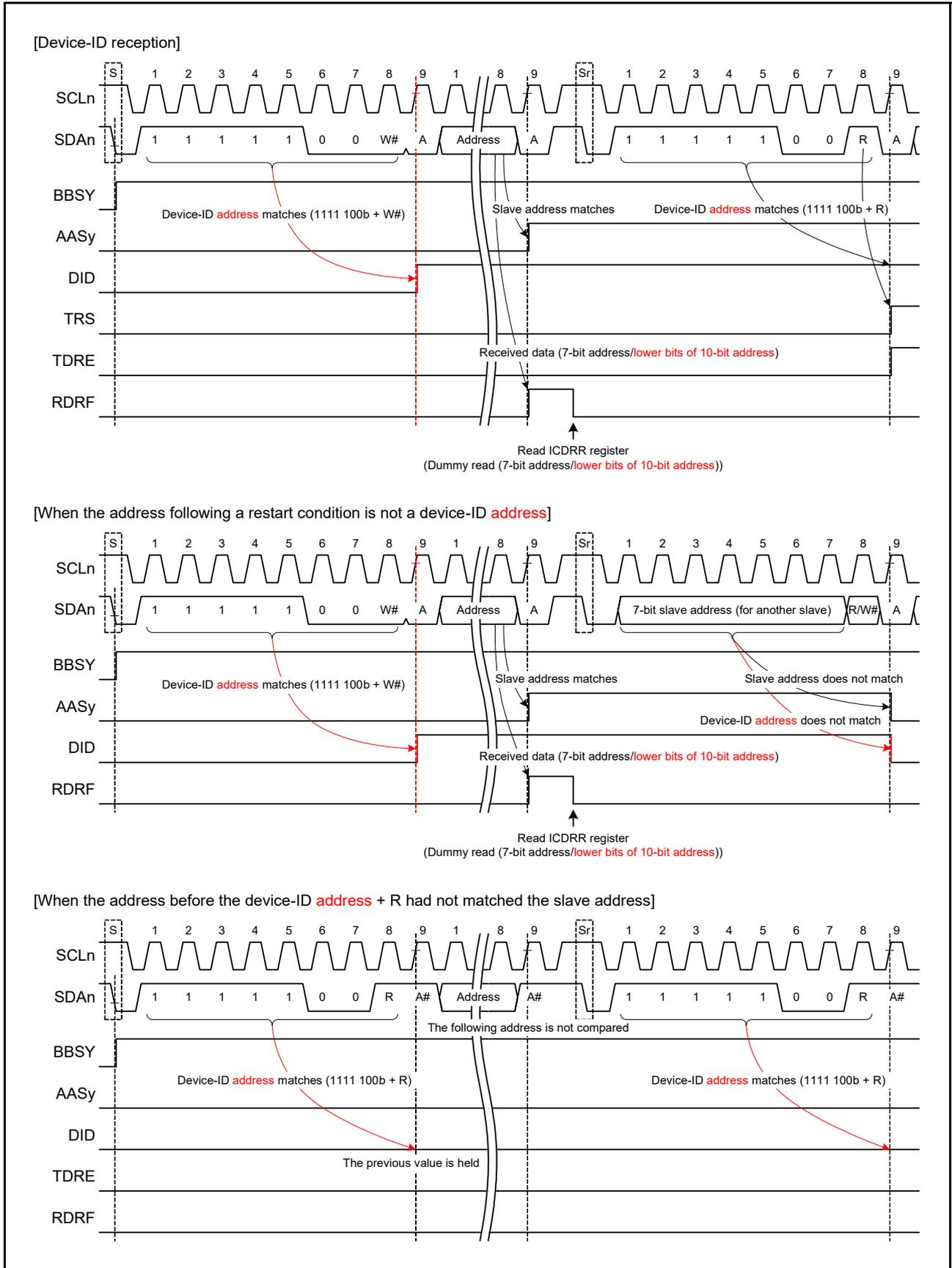
Figure 31.28 Set/Clear Timing of the AASy and DID Flags during Reception of Device-ID Address
