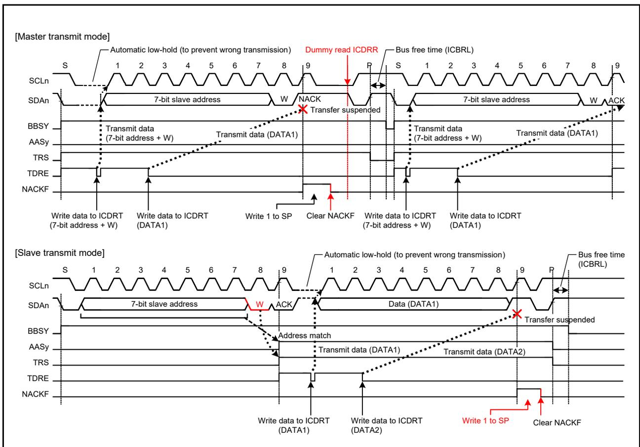
Figure 31.31 Suspension of Data Transfer when NACK is Received (NACKF = 1)
