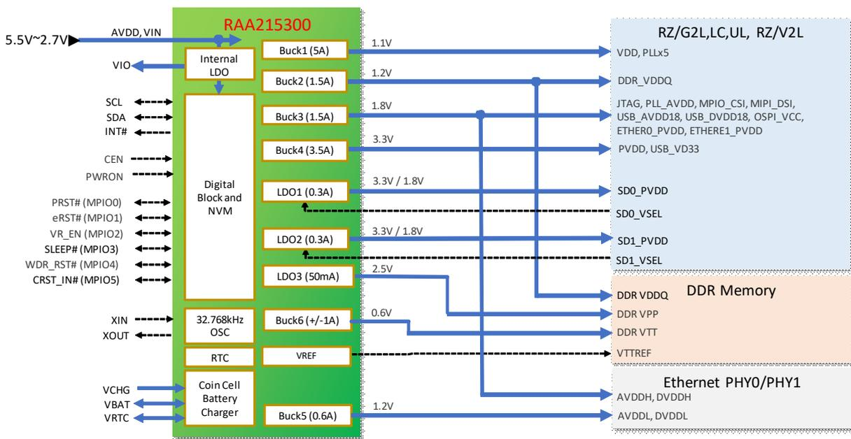
Figure 1. Typical Application Diagram - MPU Power
