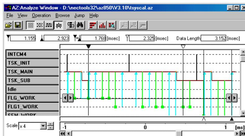
Figure 7-2 Image of Realtime OS Task Analyzer
