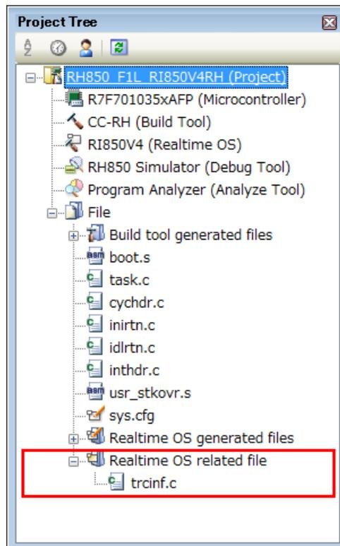
For the trace information file, select [Ignore re-compiling/assembling the source file] for [Handling the source file includes non-existing file] under [Build Method] on the [Property] panel of the CC-RH build tool.
