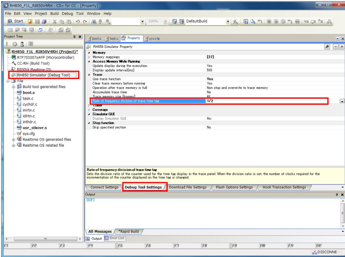
And turn on the trace function of the debugger(press the icon of a footprint mark).
