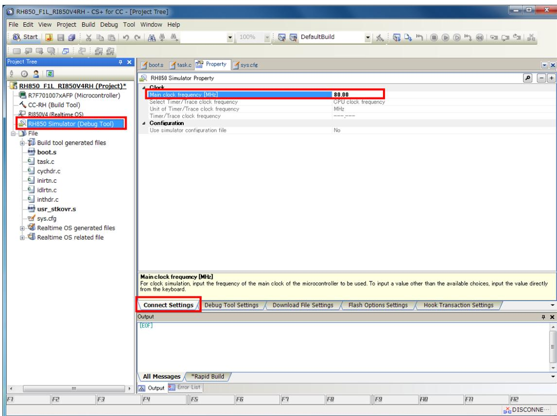
figure 9-12 [debug Tool] Tab in The property of RH850 Simulator(debug tool RH850)
