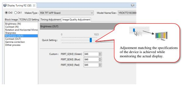
Figure 1: Image quality adjustment screen (brightness (OUT))
