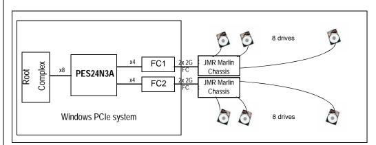
Figure 4 FC Throughput Measurement Setup with the PES24N3A
