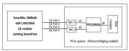
Figure 2 GE Throughput Measurement Setup with the PES24N3A
