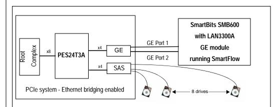
Figure 11 SAS Throughput Measurement Setup with the PES24N3A
