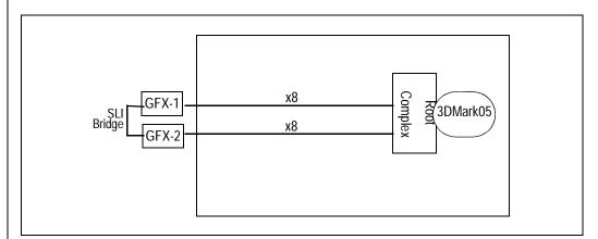
Figure 9 Graphics Setup Using 3DMark, without PES24N3A
