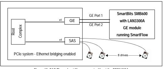
Figure 12 SAS Throughput Measurement without the PES24N3A
