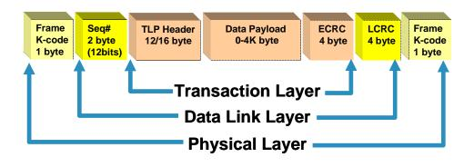
Figure 1 Framing Overhead in a Typical Transaction Packet
