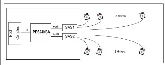
Figure 6 SAS Throughput Measurement Setup with the PES24N3A
