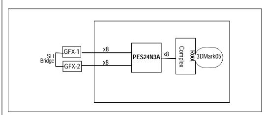
Figure 8 Graphics Setup Using 3DMark, with PES24N3A
