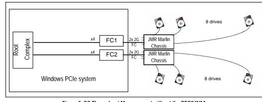
Figure 5 FC Throughput Measurement without the PES24N3A
