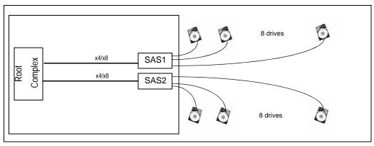
Figure 7 SAS Throughput Measurement without the PES24N3A using x4 SAS Connections
