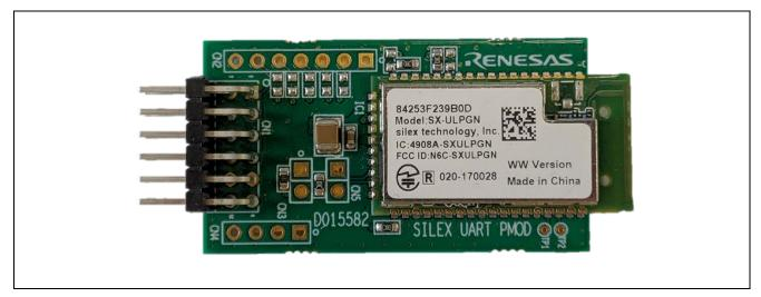
Figure 1. Wi-Fi Pmod™ Expansion Board
