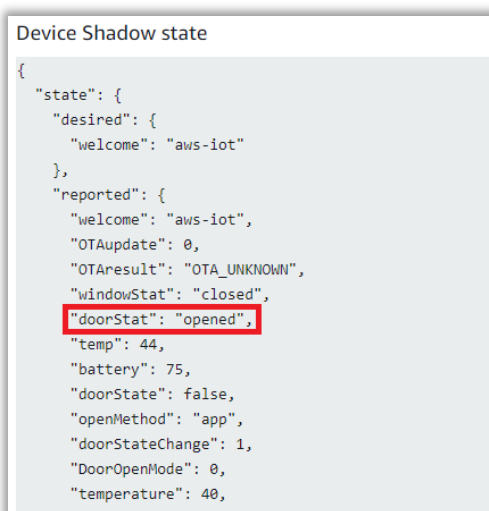
Figure 54. Shadow state when door is open
