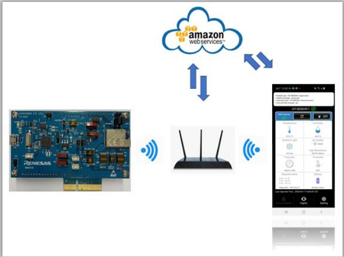
Figure 51. Architecture of AWS IoT
