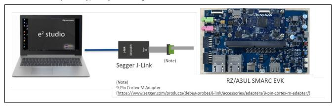
Figure 26: System Configuration Example - SMARC EVK
