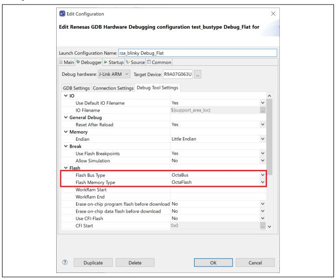
Figure 100: Flash related settings in Debug Tool Settings
