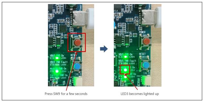
Figure 31: LED Status after Turning on EVK
