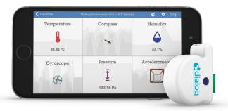
and environmental sensors. All this on a board measuring just 16 x 15 mm.
