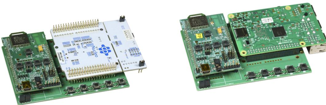
Dialog offers two OpenD development kits for either the fixed, hub part (FP) or the portable, client part (PP). The HW of the kit comes with a Cordless Voice Module (CVM), with a plugin option for a Raspberry Pi (RPI) or a Nucleo development board. For the kit software is available by means of a DECT stack together with application software. Simply download the OpenD software from the DECT Forum website, where you'll also find an online tutorial and code snippets.
