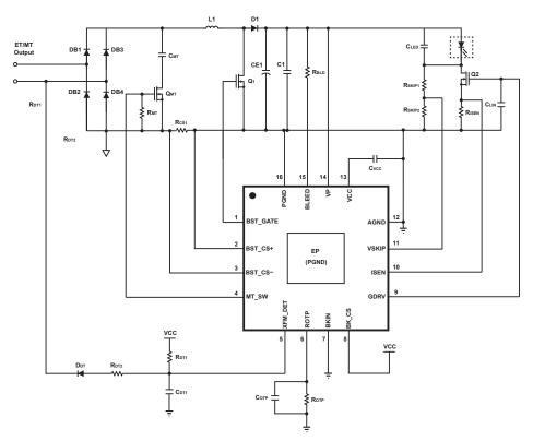
Figure 3.2 : Typical Schematic for 38V/105mA (4W) Boost-Linear Configuration
