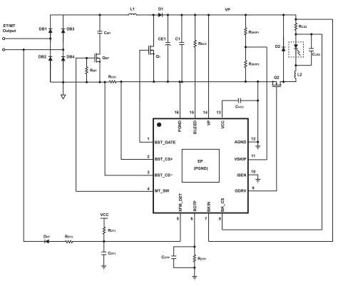
Figure 3.1 : Typical Schematic for 12V/350mA (4W) Boost-Buck Configuration
