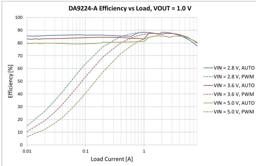
Efficiency Diagram DA9224-A, measured using 2520 size inductor with Typ. 8 mOhm DCR
