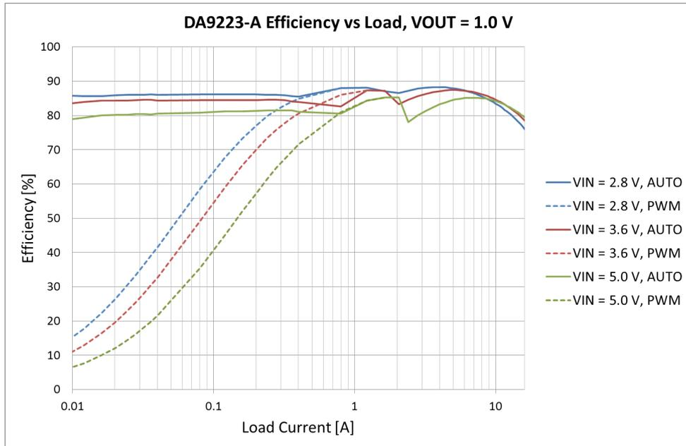
Efficiency Diagram DA9223-A, measured using 2520 size inductor with Typ. 8 mOhm DCR
