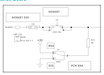
**Figure 28: Power Commander Switches**
