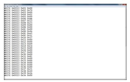
Figure 29: Register Dump (.txt File) Example
