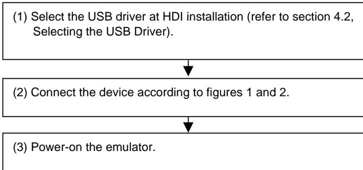
**Figure 6 Setup Procedures**
