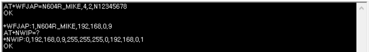
Figure 18: Debug Console – Connect to AP
