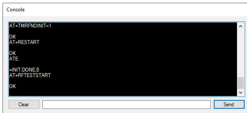
Figure 9: Debug Console – TX Mode
