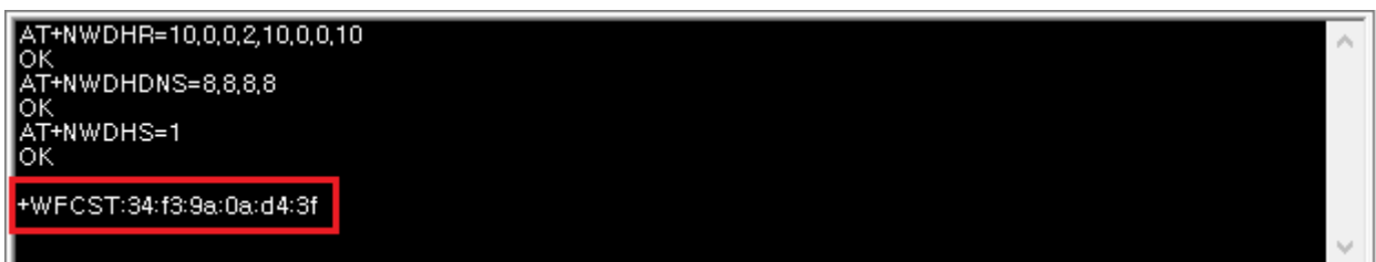
Figure 23: Debug Console – DHCP Configuration
