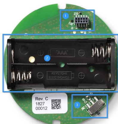
Figure 4: PCBA of DA14585 IoT MSK: Bottom View
