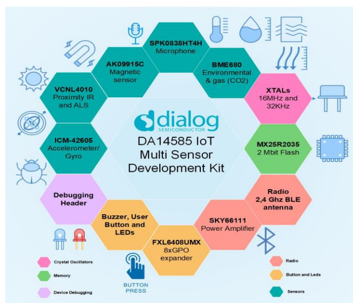
Figure 2: DA14585 IoT MSK Block Diagram
