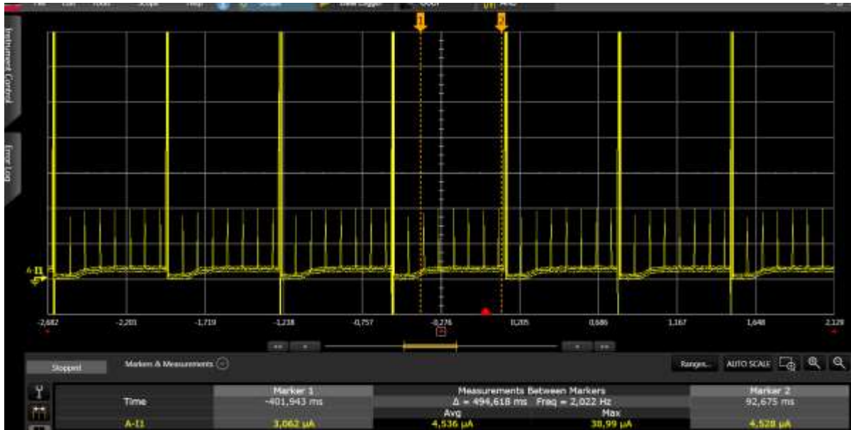
Figure 31: Average Current During Extended Sleep Mode
