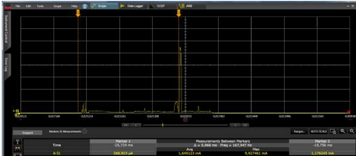
Figure 30: Peak Current During a BLE Connection Event
