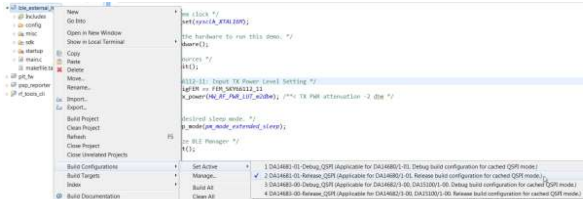
Figure 23: Set Build Configuration
