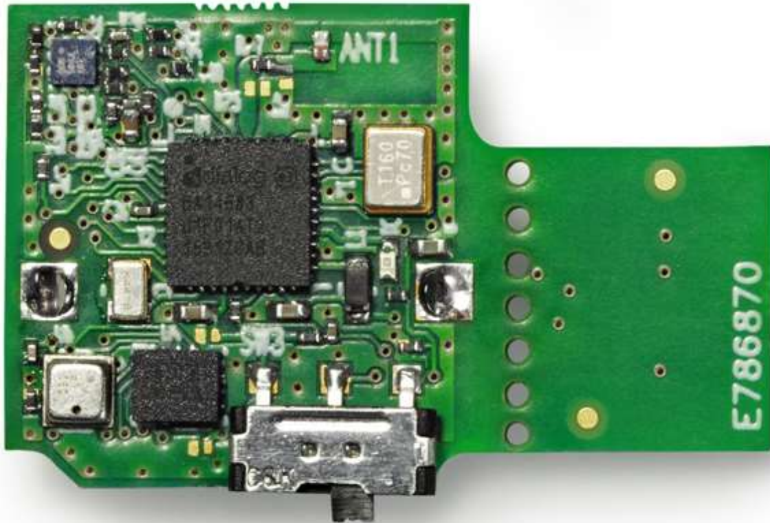
Figure 11: IoT Sensor reference board (top view)
