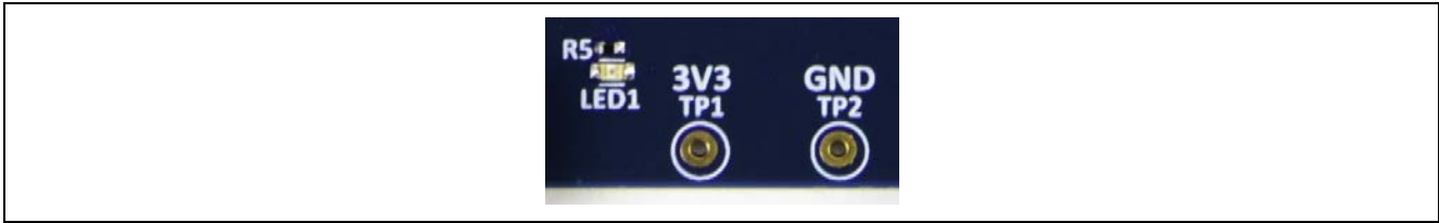
Figure 7. TP1, TP2, and LED1 on the Target Board
