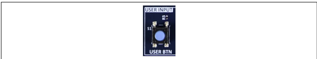
Figure 16. User Switch (S1) on the Target Board
