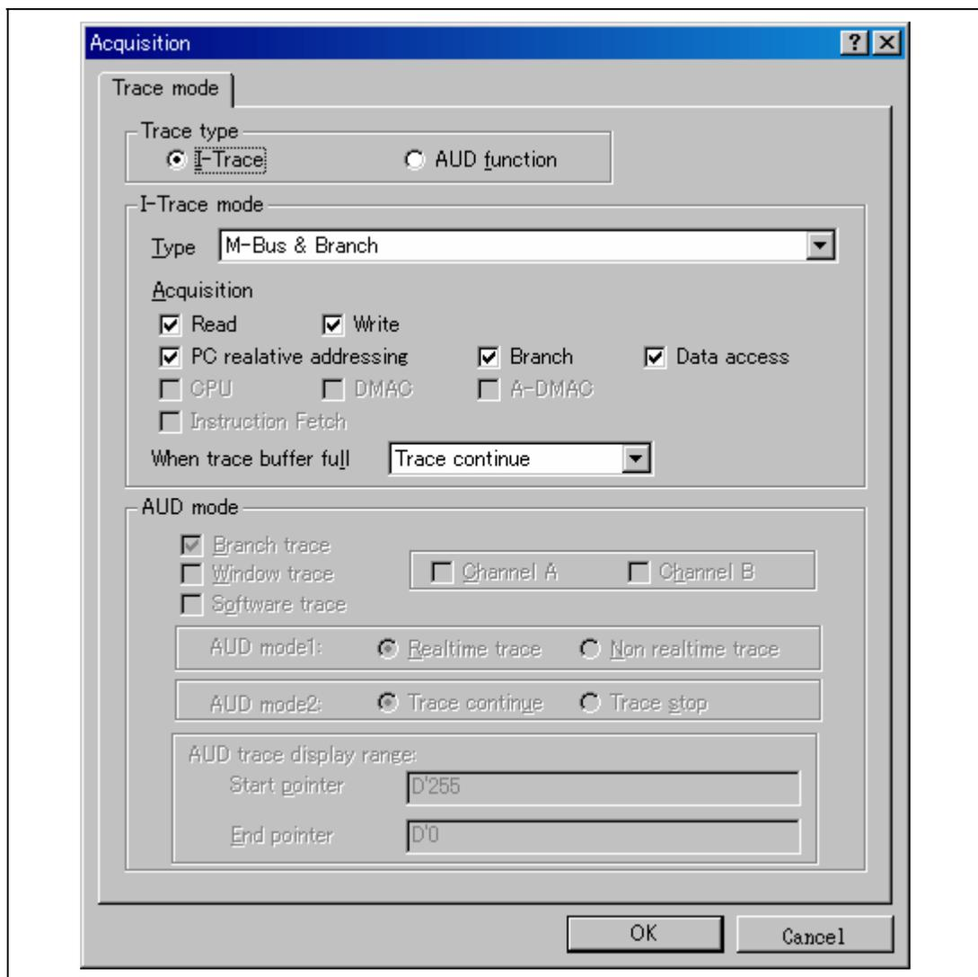
**Figure 2.2 [Acquisition] Dialog Box – Internal Trace Function**
