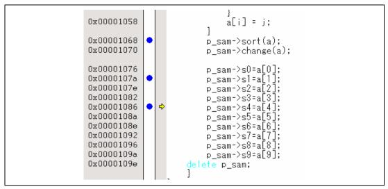
Figure 2.1 [Source] Window at Execution Halted (Sequential Break)
