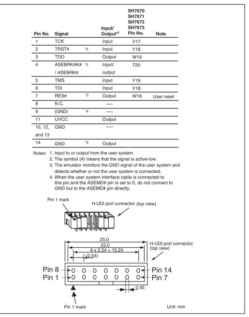
Figure 1.1 Pin Assignments of the H-UDI Port Connector (14 Pins)
