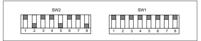
Figure 4.1 DIP Switch Setting at Shipment
