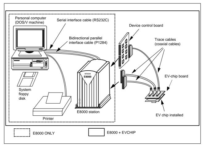
Figure 2.1 Test System Configuration
