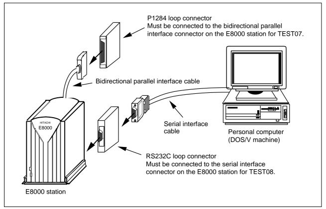
Figure 4.2 Loop Connector Installation
