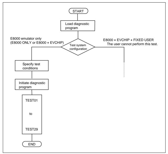
Figure 3.1 Diagnostic Program Operation Flowchart
