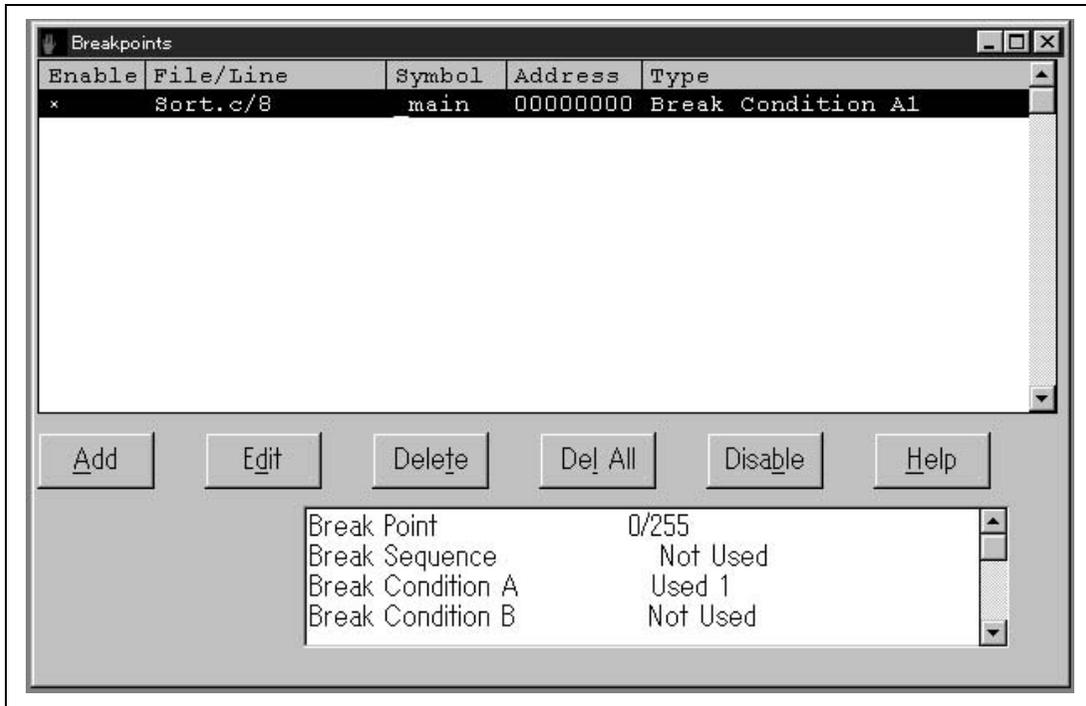
**Figure 3.41 [Breakpoints] Window ([Break Condition A] Setting)**
