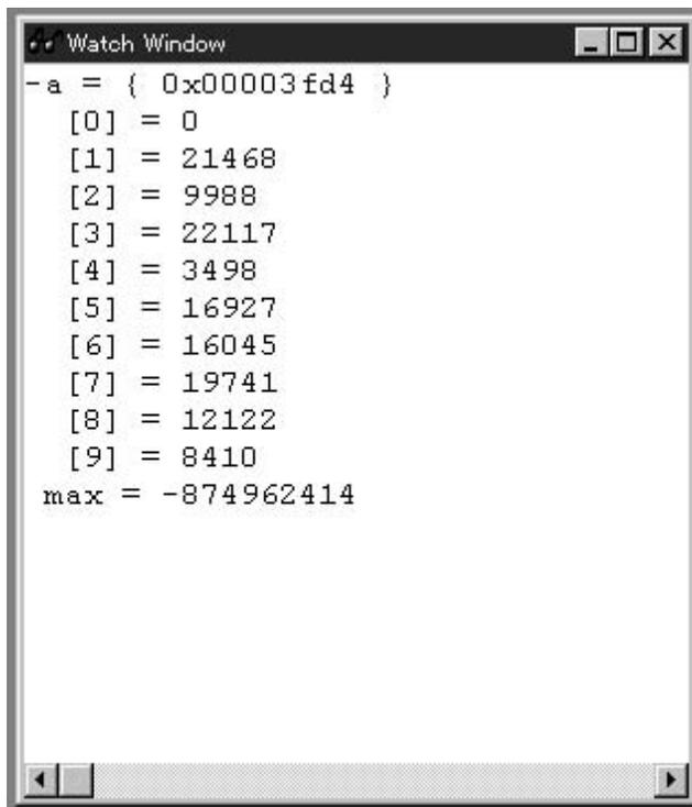
**Figure 3.25 [Watch] Window (Displaying Array Elements)**
