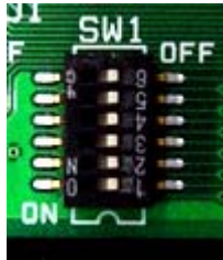
Figure 2 Switch for Masking Signals
