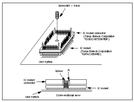
Figure 4 Fastening IC Socket Connector
