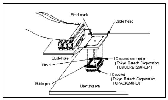
Figure 5 Connecting User System Interface Cable to User System
