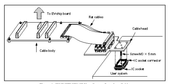
Figure 1 HS 7055ECF81H User System Interface Cable
