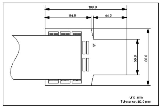
Figure 7 Dimensions for User System Interface Cable Head
