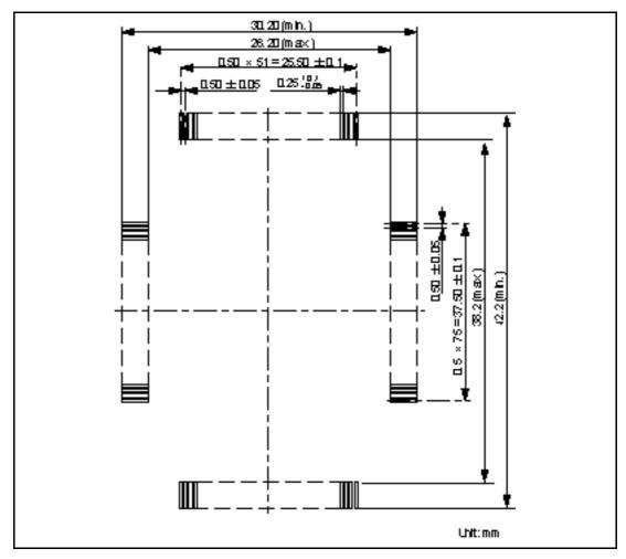
Figure 6 Recommended Dimensions for Mount Pad
