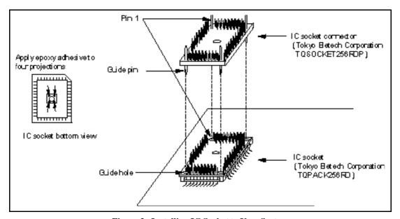
Figure 3 Installing IC Socket to User System
