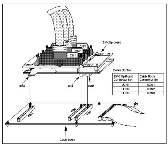
Figure 2 Connecting User System Interface Cable to EV-Chip Board
