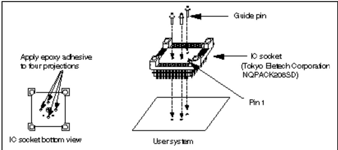
**Figure 3 Installing IC Socket to User System**
