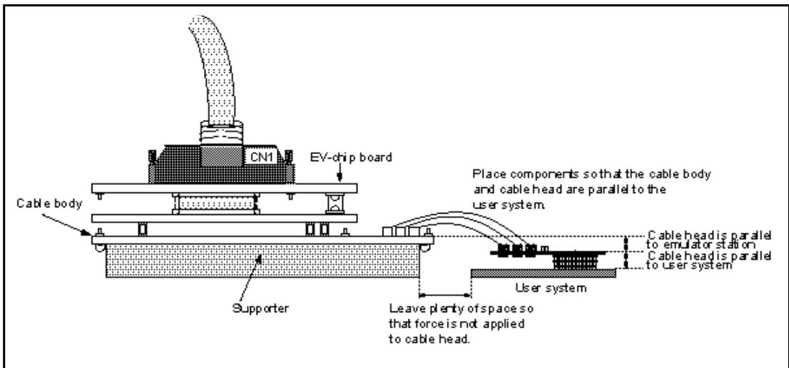
**Figure 9 User System Interface Cable Location Example**
