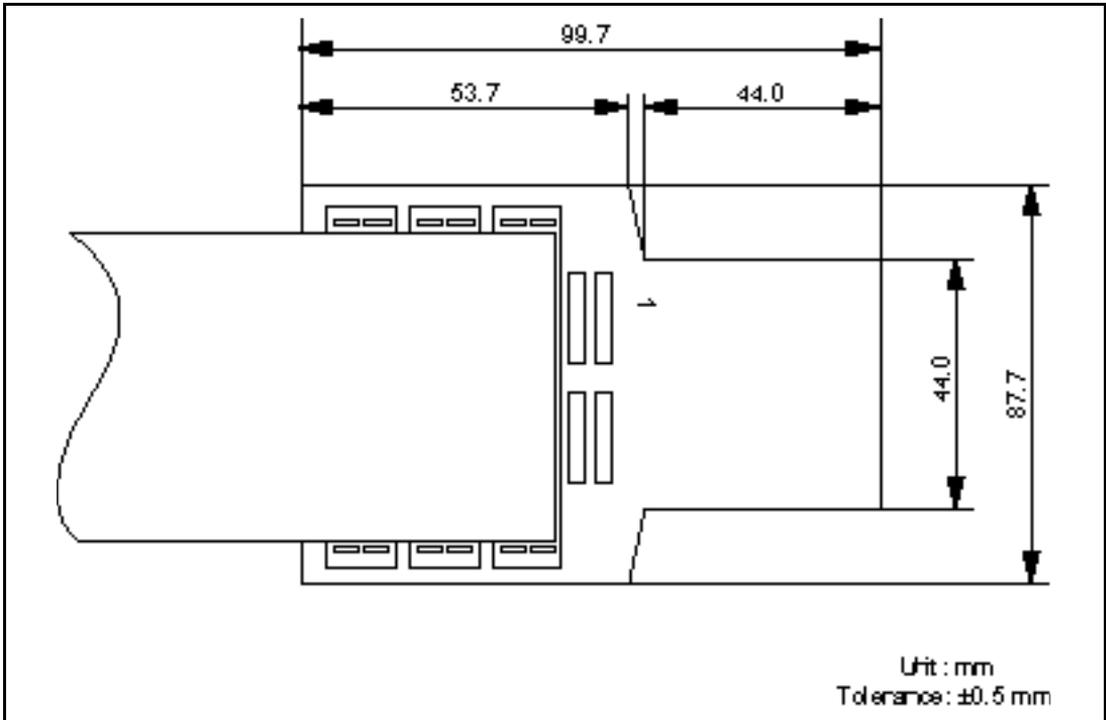
Figure 6 Dimensions for User System Interface Cable Head
