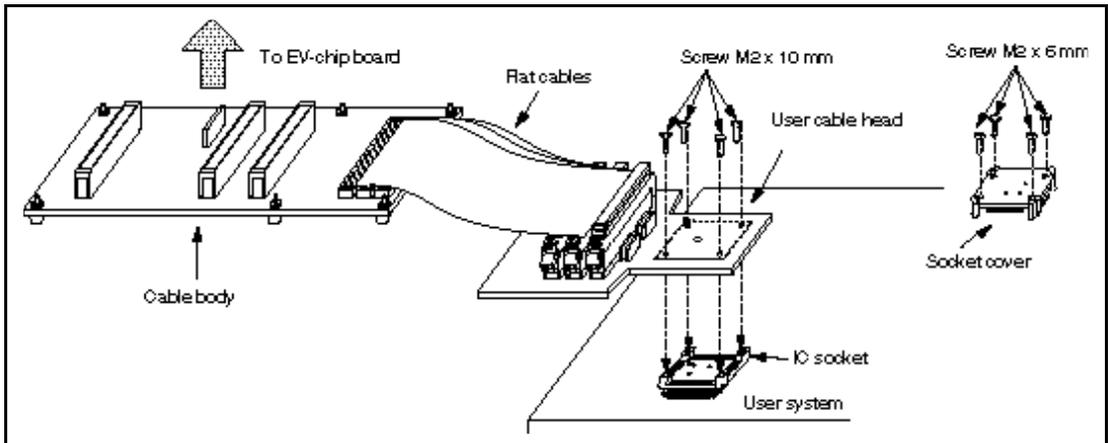
Figure 1 HS 7054ECH8 1H User System Interface Cable
