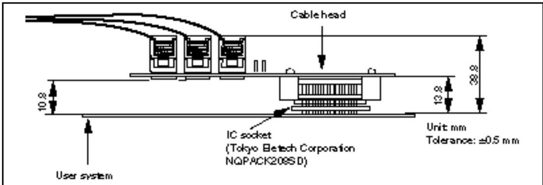
Figure 7 Resulting Dimensions after Connecting User System Interface Cable
