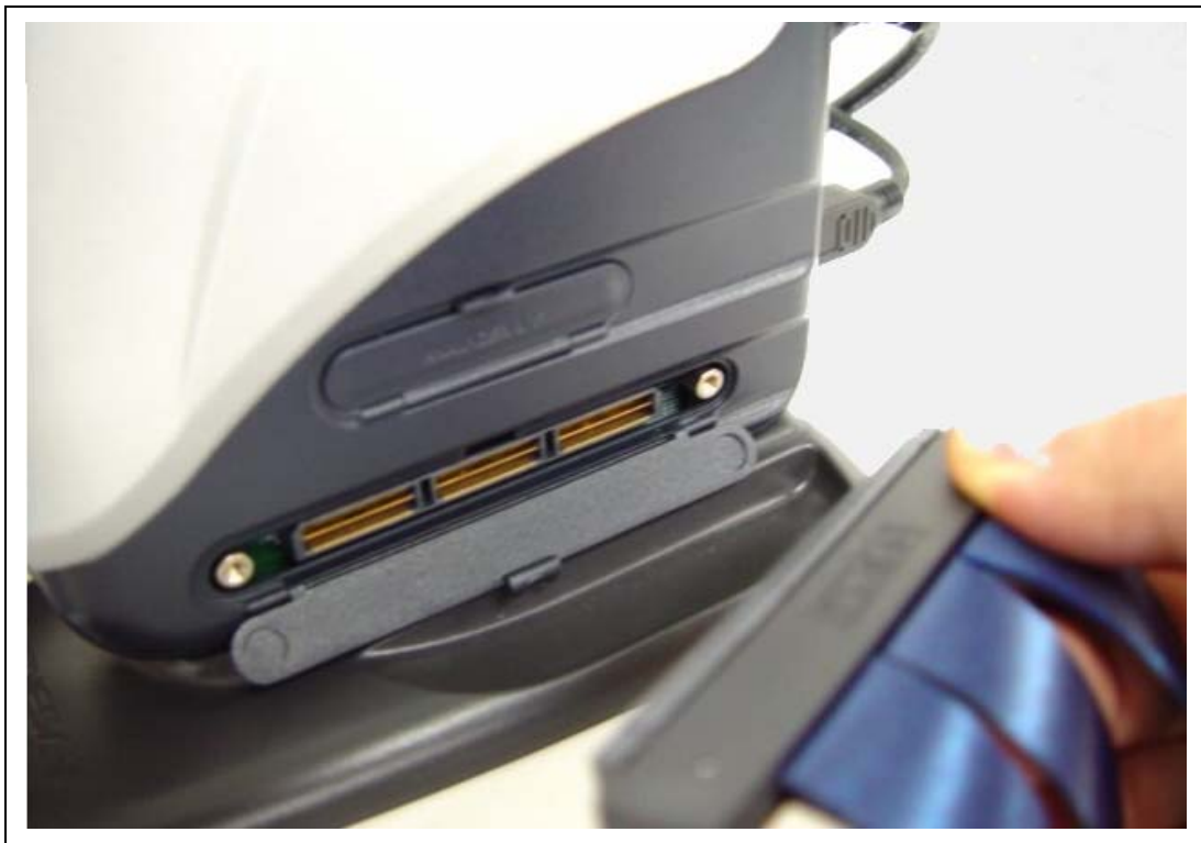
Figure 2.19 Connecting the Trace Cable to E200F
