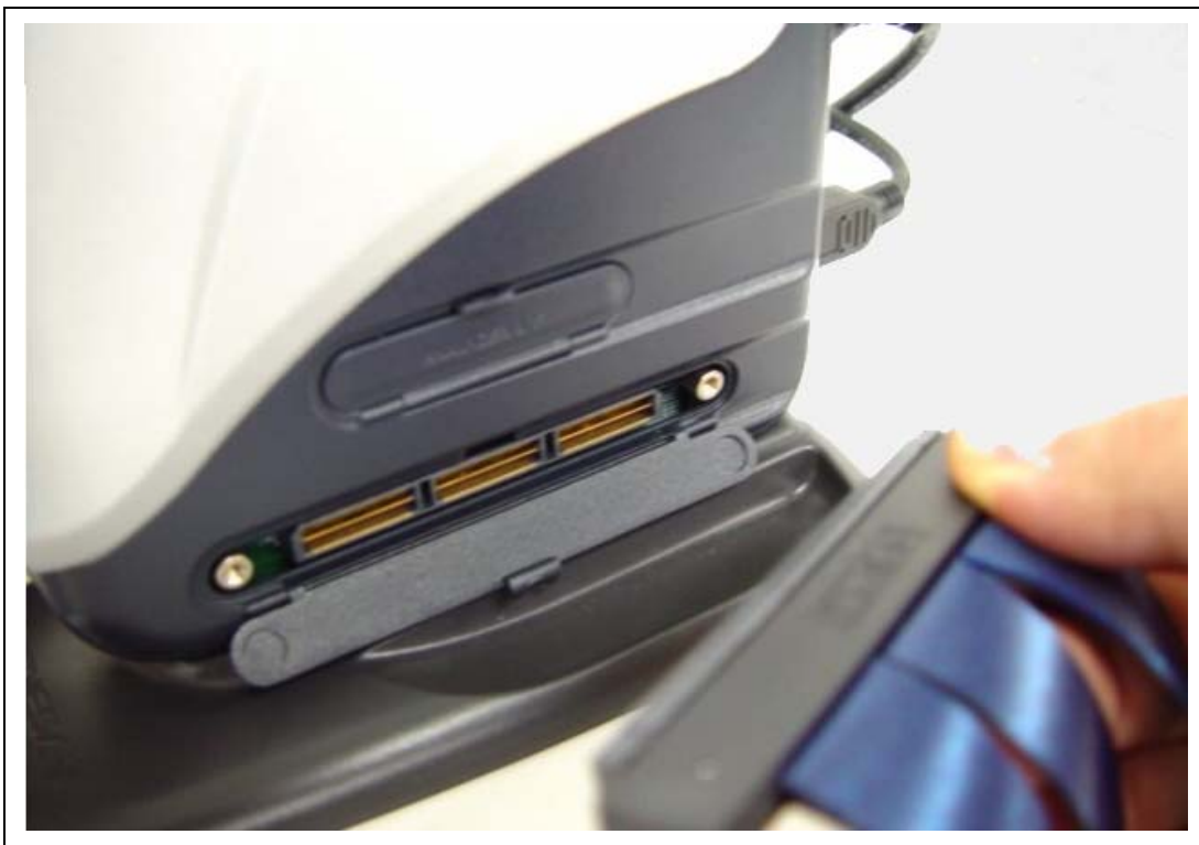
Figure 2.16 Connecting the Trace Cable to E200F
