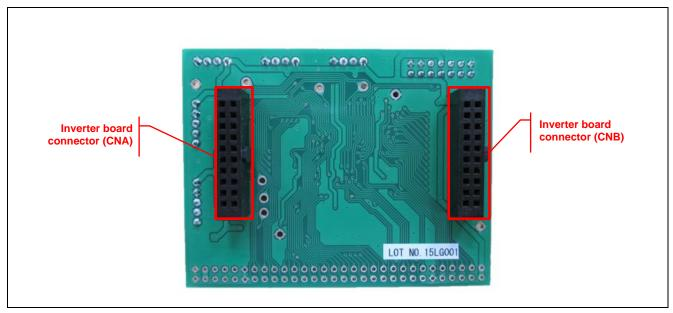
Figure 3.2 RX24T CPU Card Layout (Bottom view)
