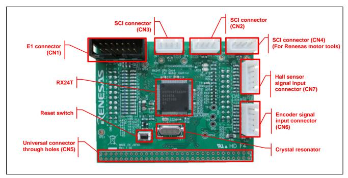
Figure 3.1 RX24T CPU Card Layout (Top view)
