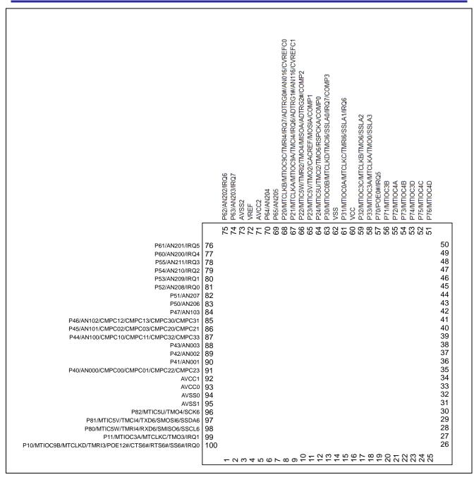
Figure 6.2 RX24T Pin Assignments (2/2)
