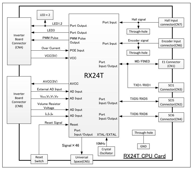
Figure 2.1 RX24T CPU Card Block Diagram
