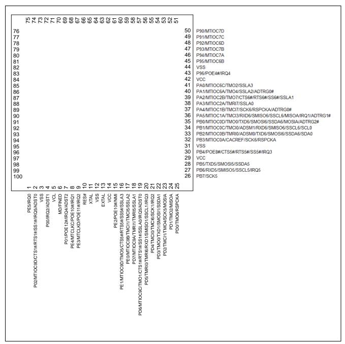
Figure 6.1 RX24T Pin Assignments (1/2)
