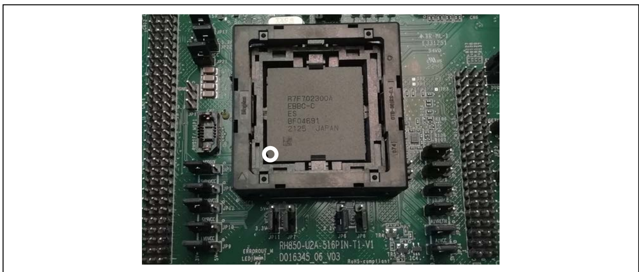
Figure 1.13 Enplas OTP-516(961RS)-0.8-048S-00 socket with mounted device
