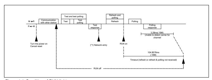
Figure 4.1 Condition of RUN light on
