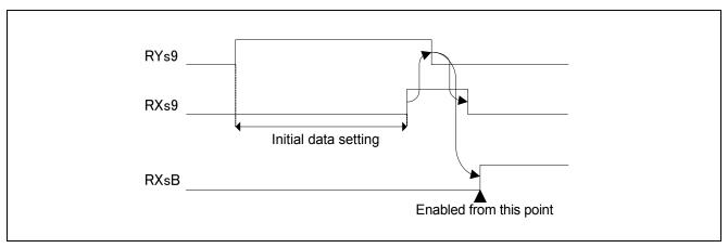
Figure 8.3 RXs9/RYs9 (initial data setting complete / setting request flag)
