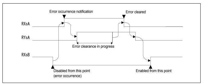
Figure 8.5 RXsA/RYsA (error status / reset request flag)
