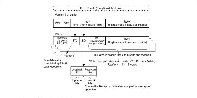
Figure 9.3 Details of SQ value (M→R data)
