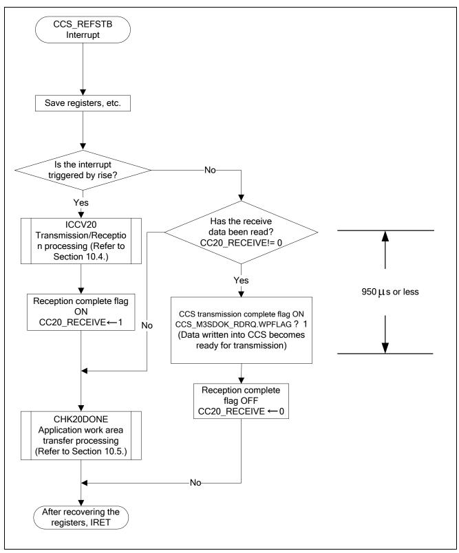
Figure 10.2Transmission/Reception Processing Using Interrupt (CCS\_REFSTB signal)
