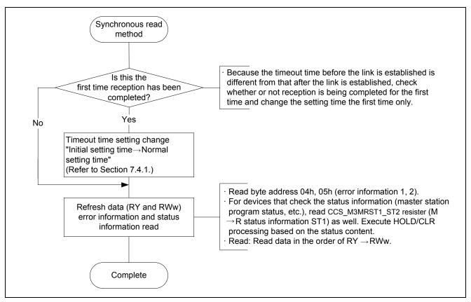
Figure 7.4 Synchronous Read Method
