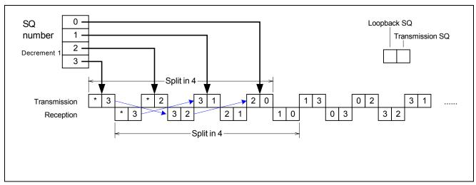
Figure 9.5 Details of SQ value(loopback)
