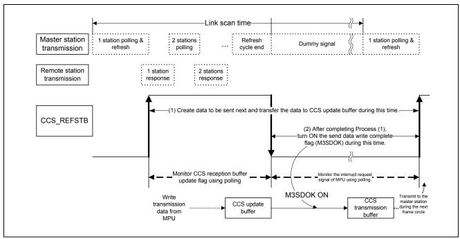
Figure 11.1Link Scan Time and CCS\_REFSTB Signal Change
