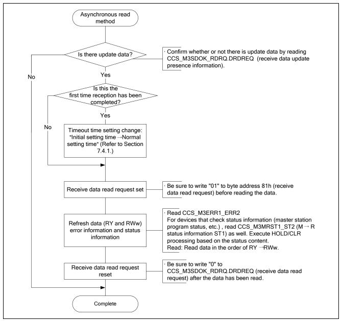
Figure 7.5 Asynchronous Read Method
