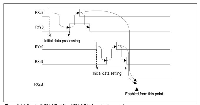
Figure 8.4 When both RXs8/RYs8 and RXs9/RYs9 are implemented
