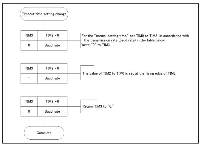
Figure 7.8 Normal Setting Time → Initial Setting Time
