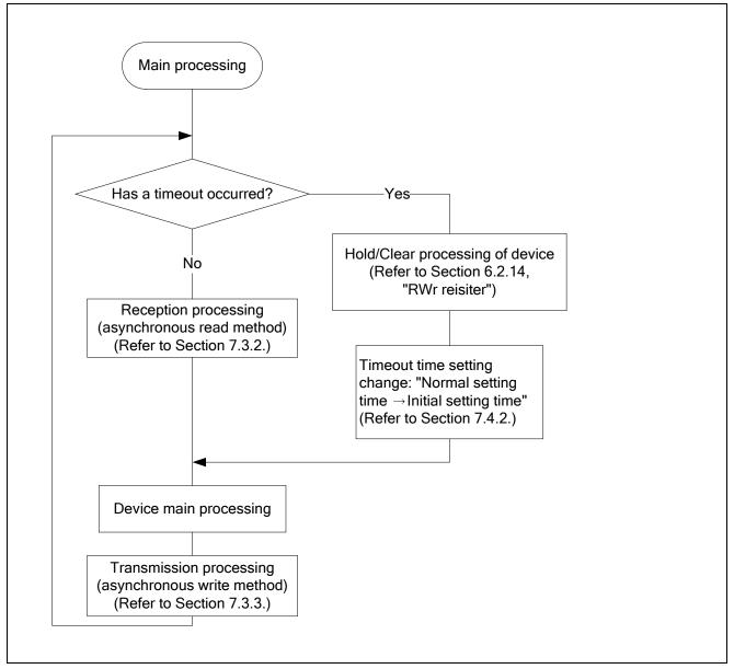
Figure 7.3 Asynchronous Read Method / Asynchronous Write Method
