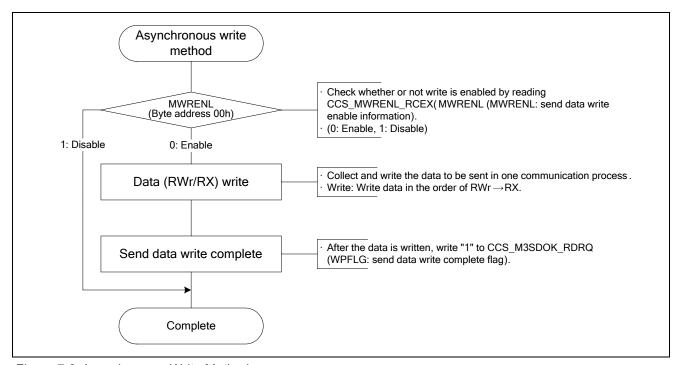
Figure 7.6 Asynchronous Write Method
