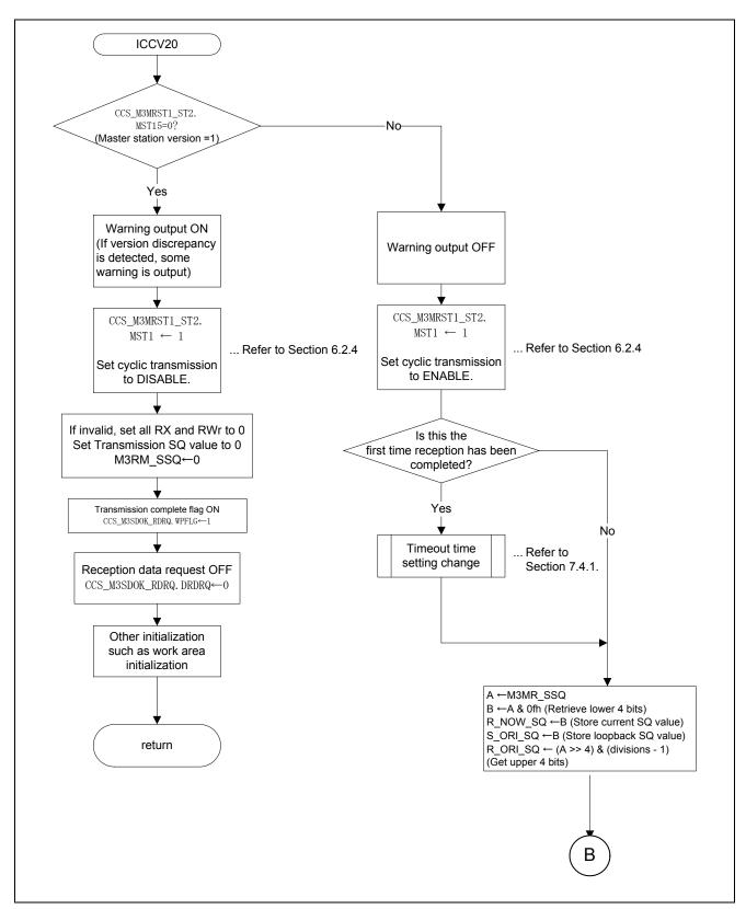
Figure 10.4Transmission/Reception Processing Module (ICCV20)
