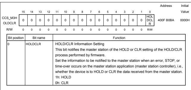
Caution The HOLD/CLR process holds or clears data received from the master station when an error, STOP, or timeout occurs on the master station application (master station controller).
