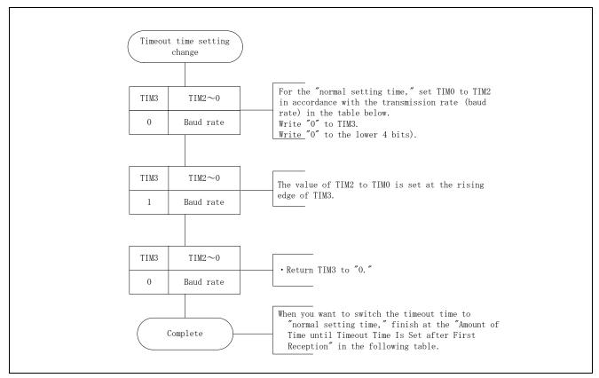
Figure 7.7 Initial Setting Time → Normal Setting Time
