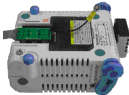
Figure 2-5. Connect the QB-RL7811A to the probe
