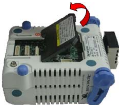
Figure 2-1. Acrylic Board Removal Method
