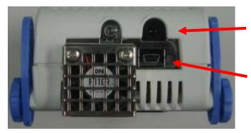
Power supply connector (Connect AC adapter)
