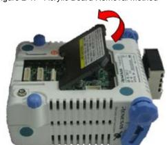
Figure 2-1. Acrylic Board Removal Method
