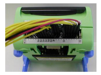
Figure 2-9. Connection of QB-78K0SKX1 (40-pin 2.54 mm pitch connecter) to Target System
