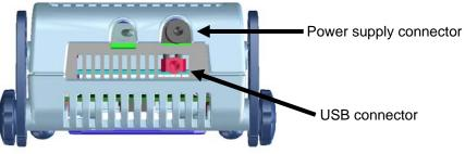
Figure 1-1. Names of Parts of QB-78K0FX2L
