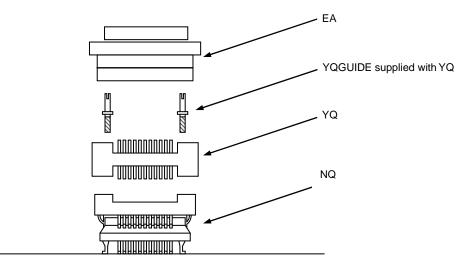
Figure 2-4. Mounting of EA, YQ and NQ
