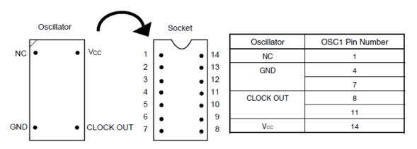
Figure 2-3. Mapping of Oscillator to Socket
